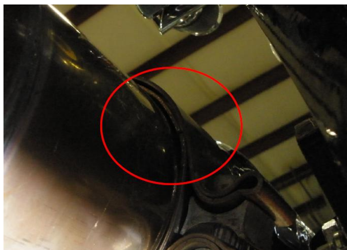
Fig. 7: Muffler Clamp covers inboard seal slot profile
