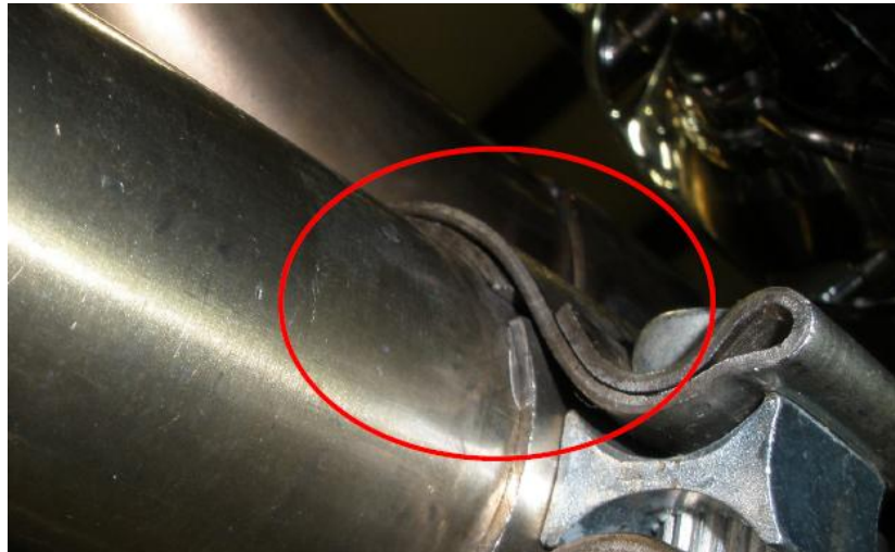
Fig. 6: Headpipe Clamp covers inboard seal slot profile
