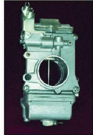
**Both the Mikuni HSR42 and HSR45 carburetors have their advantages. The 42 (top) is easier to install while the 45 can deliver more peak**
